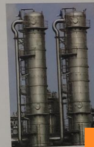
▲ Figure 3 A distillation tower crude oil is separated into fractions. The oil is heated to about 400 °C. Hydrocarbon gases rise up the tower and condense at different levels on their boiling points.
